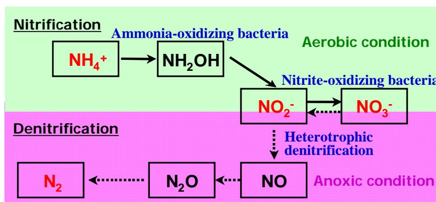
**Figure 1.1** Schematic diagram of biological nitrogen removal pathway.
