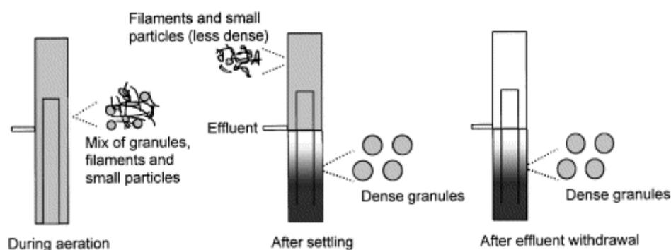
**Figure 1.5** Selection of well-settling, dense granules by setting a short settling time (Beun et al., 2002).
