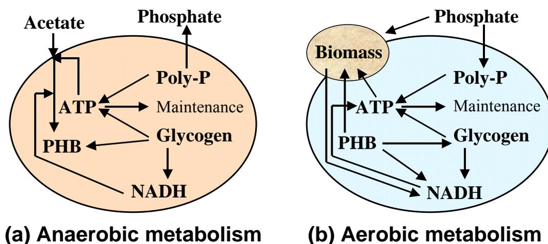
**Figure 1.2** Schematic diagram of metabolisms of PAOs. (De Kreuk, 2006).
