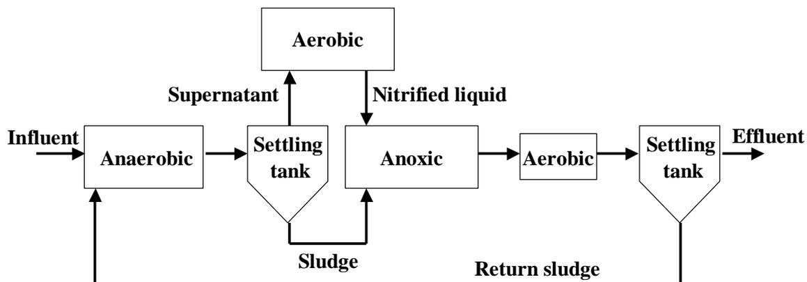
**Figure 1.3** Schematic diagram of external nitrification (DEPHANOX) process.
