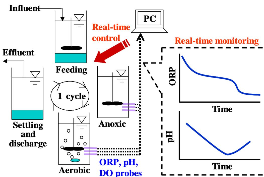
Figure 1.4 Schematic diagram of real-time control strategy in BNR.
