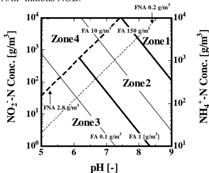
**Figure 1.4** Dependence of free ammonia (FA) and free nitrous acid (FNA) on pH in the solution proposed by Anthonisen *et al.* (1976). Zone 1 shows FA inhibition of *Nitrobacter* and *Nitrosomonas*, Zone 2 shows FA inhibition of only *Nitrobacter*, Zone 3 shows complete nitrification, and Zone 4 shows FNA inhibition of *Nitrobacter*. Symbols: solid lines, FA of 0.1, 1, 10 and 150 mg l<sup>-1</sup>, respectively; dotted lines, FNA of 0.2 and 2.8 mg l<sup>-1</sup>.
