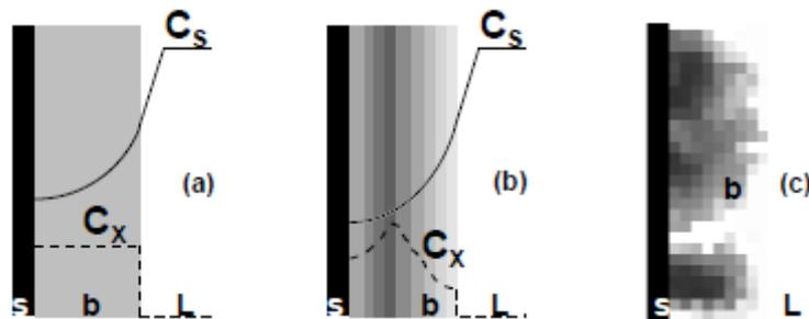
**Figure 1.1** Evolution of biofilm models from (a) uniform biomass distribution and one-dimensional substrate gradient in the 1970's, to (b) one-dimensional stratified biomass and multispecies biofilms in the 1980's, to (c) multidimensional distribution of biomass and substrate at the end of 1990's.
