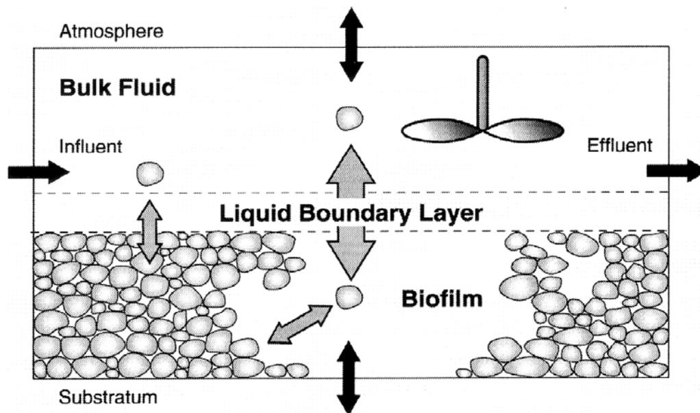
**Figure 1.2** Setup of the AQUASIM biofilm reactor compartment. Solid arrows indicate possible mass fluxes across compartment boundaries, and shaded arrows indicate mass fluxes within the compartment. Taken from Wanner *et al.* (2004).
