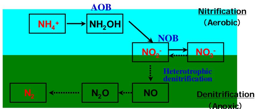
**Figure 1.5** Schematic diagram of biological nitrogen removal pathway.
