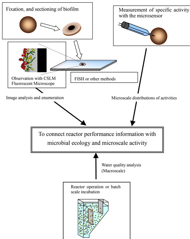
**Figure 1.6** Schematic illustration of the analysis of the *in situ* organization of a biofilm community using various methods and the connection with reactor performance (partly from Aoi, 2002).
