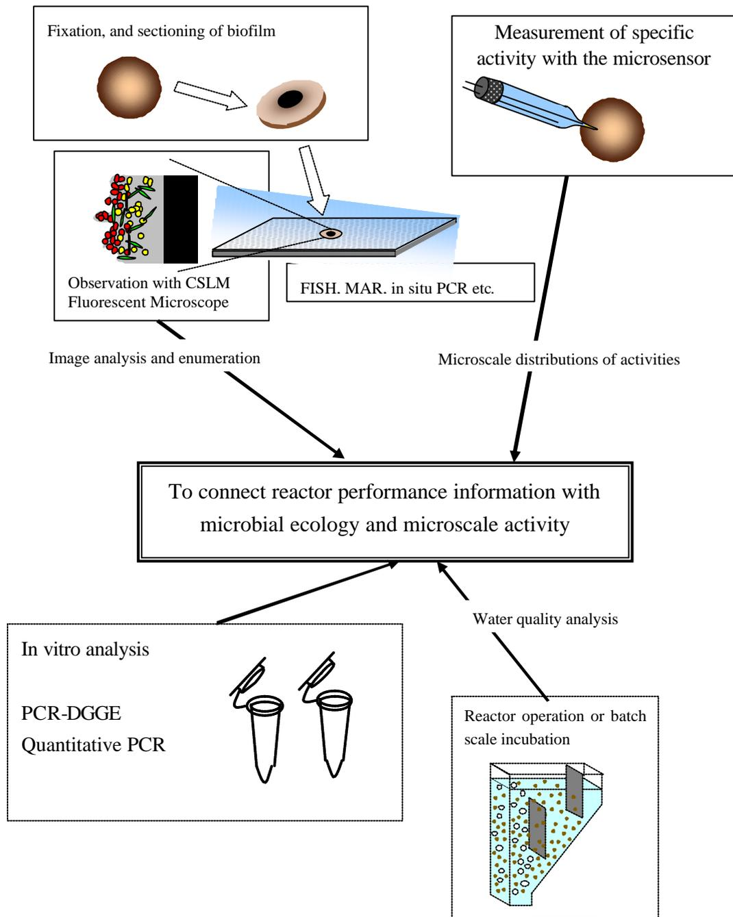
FIG. 1. Schematic for the analysis of the *in situ* organization of a biofilm community using various methods and the connection with reactor performance.
